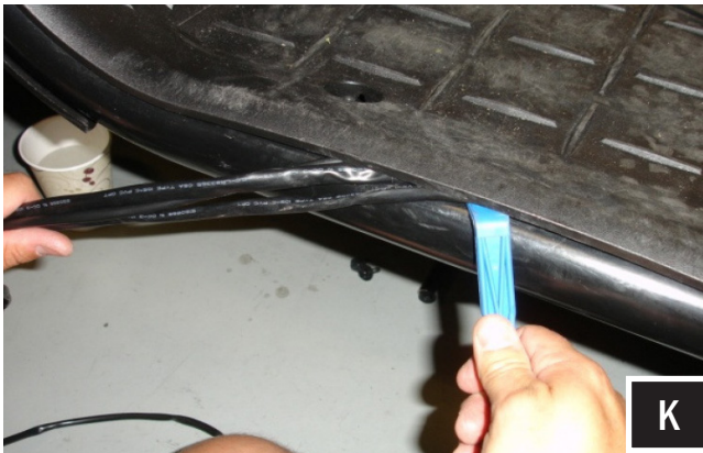
K. Route the cables along the floor to a location near the side of the driver seat to continue up the cage.
