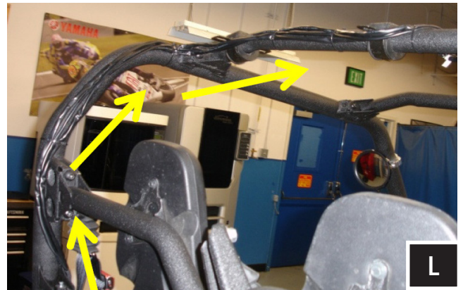
L. Run the cable up the cage (following the wires from the Overhead Stereo System).
