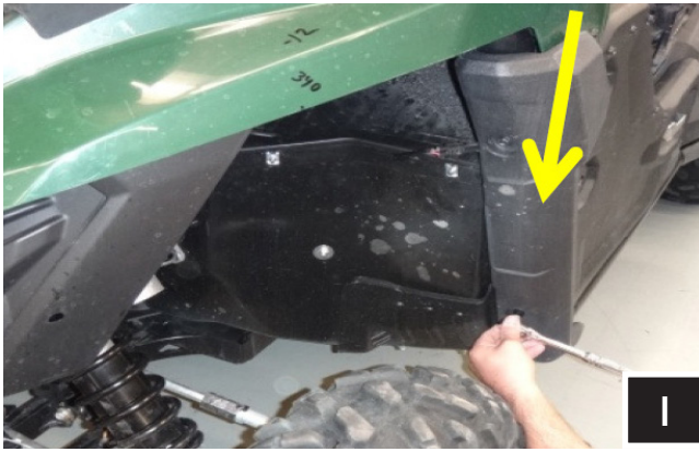
I. Remove the front wheel well protector, this is where the speaker cables will run down.
