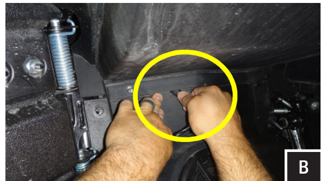
B. Gently press the floor away from the under dash and route the speaker wire harness through the floorboard joint.
