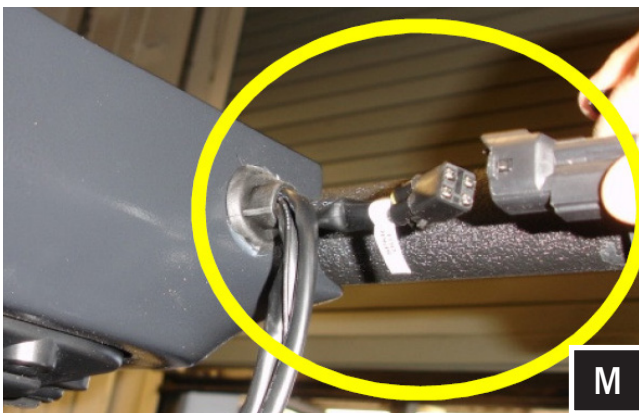
M. Locate the short output harness coming out of the main unit.
