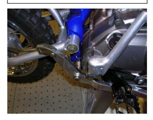
Reassemble using OEM washers and new cotter pins Items 2 and 3.
