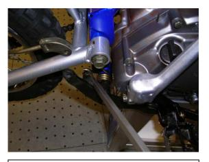
Use a large Flathead screwdriver to pry the return spring off of its perch. Remove the OEM brake lever.
