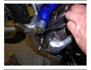
Apply a thin film of grease to pivot shaft and inside of brake lever. Slide return spring onto brake lever and install assembly on Motorcycle. Use a large zip-tie to pull the return spring onto its perch.
