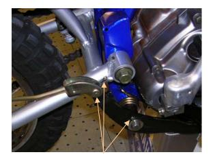
Remove cotter pins and washers from OEM brake lever pivots and retain washers for reassembly. Pull out the link pin and move linkage to the side.
