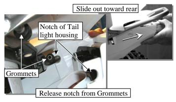
**c.** Slide the Rear Tail light housing toward rear to disconnect and release from the Rubber grommet.
