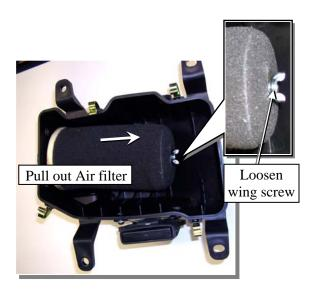
i) Loosen the Winged head screw of the Air Filter until the Air Filter can be pulled out from Air box.
