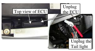
**d.** Disconnect and unplug the Tail light & the ECU located on the left side of the Filter Air box.
