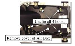
**e.** Unclip the 4 spring hooks to remove the cover of the Air box.
