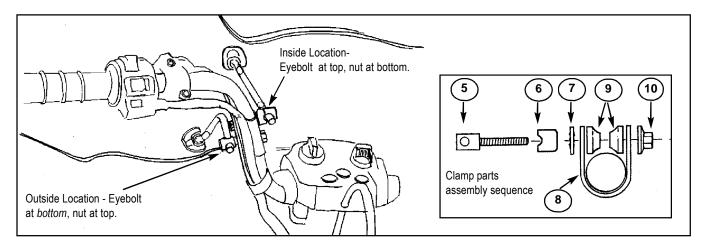
3. Mount fairing body in front of handlebar. Insert upper and lower rods into eyebolts as shown. Adjust the fairing body to be horizontal and centered in front of the headlight. The forward edge of the fairing body should be about 3/8" above the rack. Make sure the brake levers have a minimum 1/2" clearance to the fairing body.
