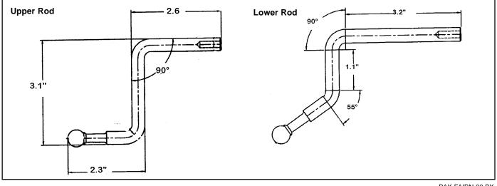
1. Support the mounting receptacle of the Fairing Body on a firm, flat surface, and firmly press ball end of upper rods into upper sockets. Ball will snap into place. Repeat for lower rods.
